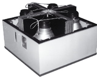
# 1559: One of the layout options of the multide-tector spectrometer module.
