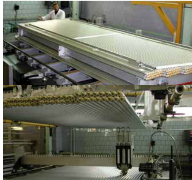
# 1639: Automatic chamber glueing machine. Chamber spacer. Glued chamber at the granite table.
