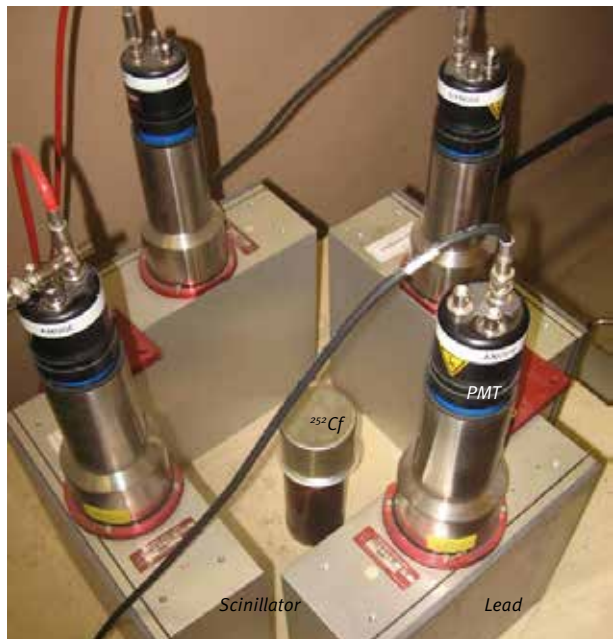
# 2978: Count of time coincidences of FM particles by PSD EJ-309 scintillators and digital technology
