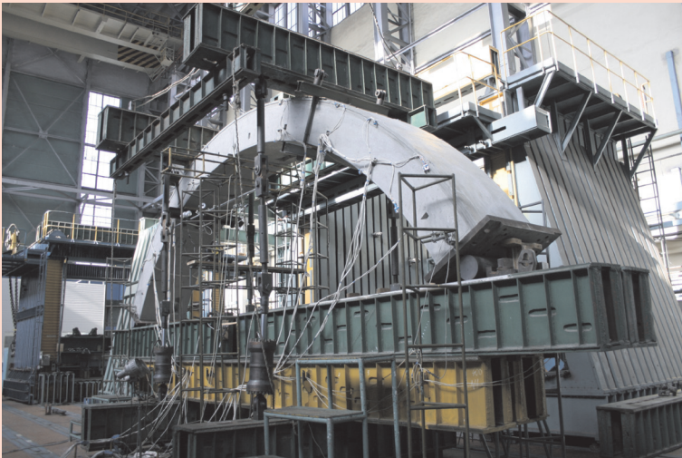
Strength tests of a tubing
