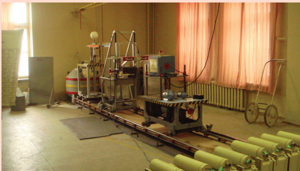
Setup for attestation of radiometric and dosimetric instruments
