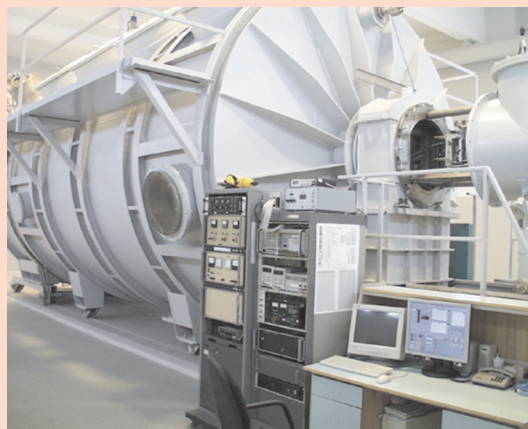
Cryogenic vacuum test bench
