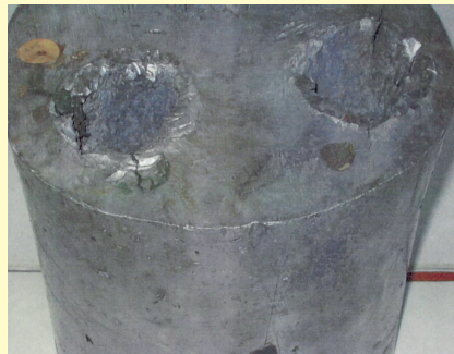
Figure 3: Craters from particle with foam layer (alloy AD-1, V_{exp} = 6.4 km/s, V_{cal} = 6.6 km/s)
