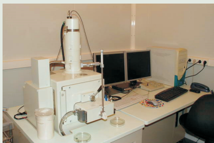
Figure 4: Electron lithographer applied at the laboratory of Project performers in combination with the JSM-6460 raster electron microscope (REM) (Jeol, Japan) equipped with an external lithographic extension NanoMaker made by the "Interface" company (Russia). It is applied to fabricate a microcircuit containing SCT nanobolometer, antenna (in which the nanobolometer is incorporated) and respective cross-connections in a single technological cycle
