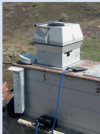
Figure 1: All-sky camera equipped with the Zeiss Distagon “fish-eye” objective ( f=30 mm, D/f = 1:3.5 ) with 180° field of view
