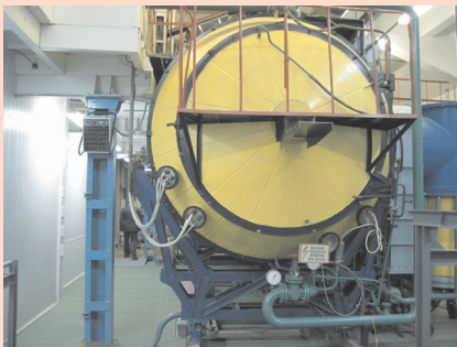
Test bench for electrophysical measurements at which processes and super-high-frequency diagnostics of a low-temperature plasma are studied
