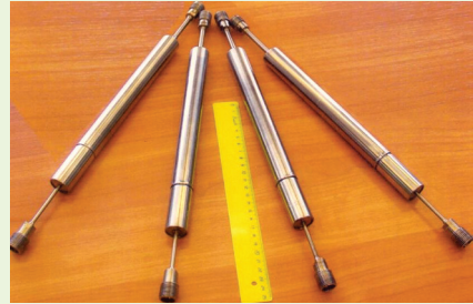
Figure 3: Evaporators with no-heat-conducting wicks
