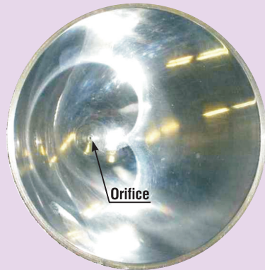
Figure 6: Laser rocket engine model with liquid injection in the paraboloid focus
