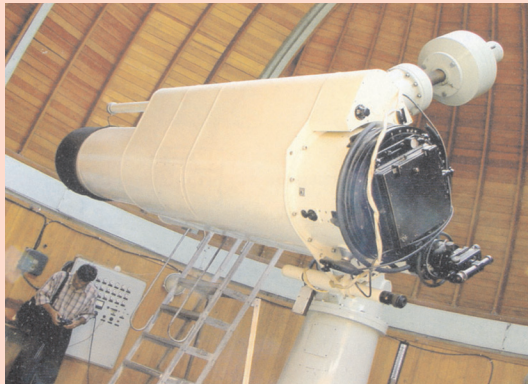
Forty-centimeter Zeiss Astrograph ( D = 400 mm, F = 2000 mm) at Gissar astronomic observatory
