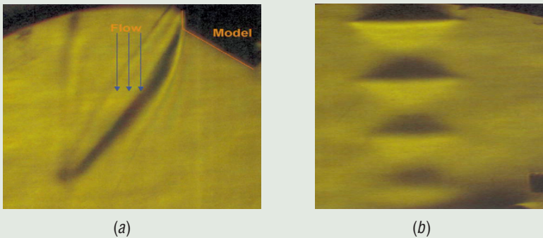
Figure 7: Density distribution in a flow around the model (a) and visualization regime demonstrating the shock wave structure in a tube (b)
