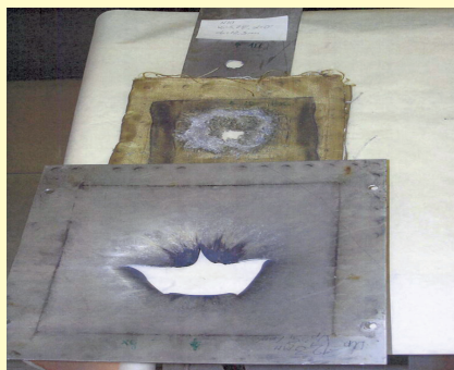
Figure 4: An experimental model with the flat shield after test
