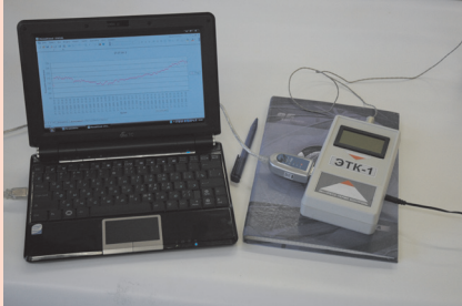
Instrument for control of volatile admixtures in thermal and energy equipment
