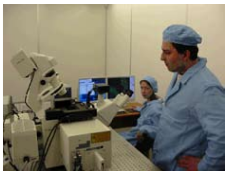
Kalvinkovskaya and Bushuk carry out investigations in advanced directions of optical nondestructive testing using a laser scanning microscope equipped with continuous wave and femtosecond lasers at the ISL in Minsk, Belarus
