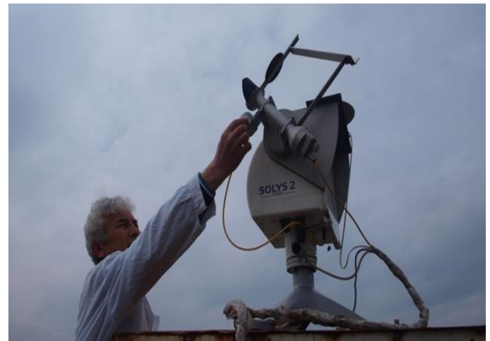
Fig.2. Complex on base of Sun tracker SOLYS-2(Kipp&Zonen)
