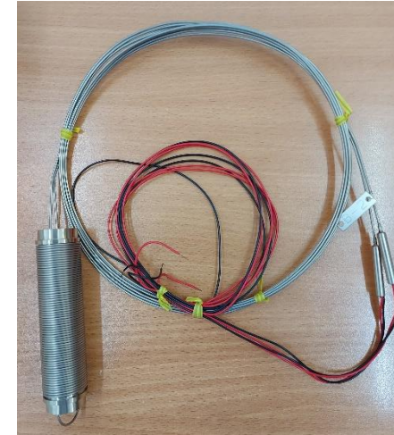
Mineral-insulated cables to be installed in the irradiation device for neutron irradiation experiment.
