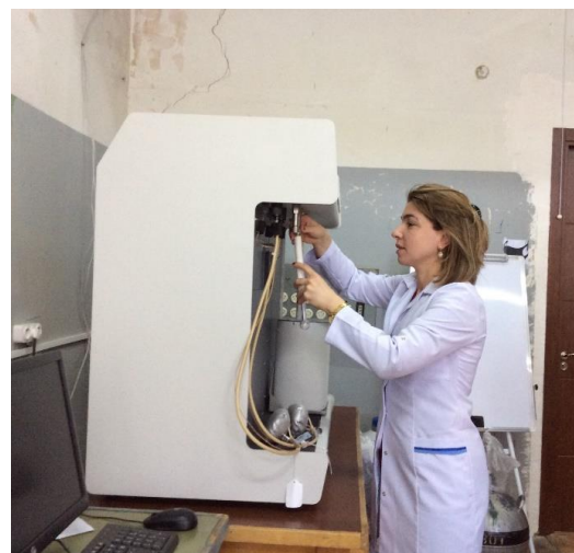
Measurements nitrogen adsorption/desorption isotherms using ASAP 2020 Plus analyzer (Micromeritics, USA) for samples of Georgian, Kazakh and Armenian
