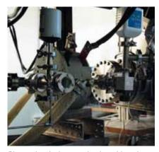
Plasmachemical reactor for deposition of extremely high-enriched 28Si isotope thin film
