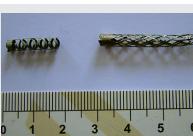
One-stage electroforming iron stents without laser cutting
