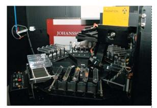
Russian made scintillating crystals used in the CMS detectors
